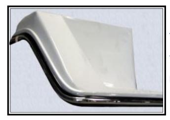
This is a sample of what a splash design looks like. Notice how we bent both the vinyl and stainless steel rubrail to fit the intricate bend details necessary for a perfect fit.
